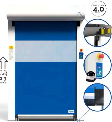
THE GLIDE K RAPID ROLL-UP DOOR is suitable for applications in supermarkets and sales points; is silent and requires little maintenance. Consist of an enclosed mantle and lower aluminium alloy bar that slides freely in the guides. The lower bar goes back into the guides in the case of accidental impact. The "K" line features a motor housed inside the winding tube, which allows installation in corridors and any other limited space, and the opening speed is increased to 2.3 m/s.
