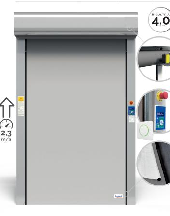
**THE PURA K-IX RAPID ROLL-UP DOOR** is characterised by the sheet sliding on grates. Designed to offer the maximum sealing for internal applications in areas where particular environmental and hygiene conditions must be maintained, such as laboratories, pharmaceutical industry buildings or food handling areas. The **"K"** line features a motor housed inside the winding tube, which allows installation in corridors and any other limited space, and the opening speed is increased to 2.3 m/s.
