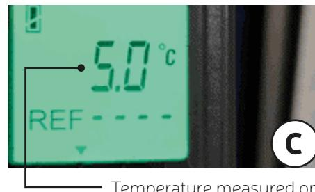
Temperature measured on the surface at risk of condensation, e.g. outer surface of door curtain
