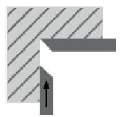
FIG. 2: chamfering for edge jointing
