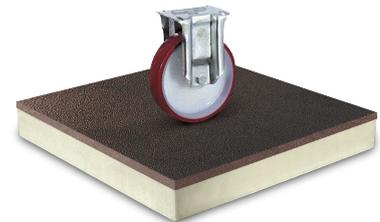
**Ceiling panels:** The panels are the same as the ones used for walls and are self-supporting for ceilings up to 4000 mm, but cannot be used to walk on or for storing materials, even temporarily. In the case of larger ceilings, i.e. when both sides of the room exceed 4000 mm, a layer of two or more panels is required; the ceiling is hung from trusses at a height of between 350 and 550 mm according to length. The suspended system is shown in pictures 8 and 9.
