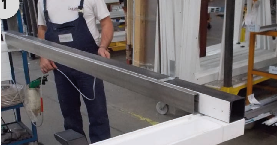
Fix the lower tubular sill to the door frame
